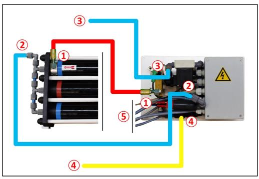
Hose for connecting the high-pressure membrane outlet to the high-pressure control valve on the back of the front panel. (Black high-pressure hose supplied)
