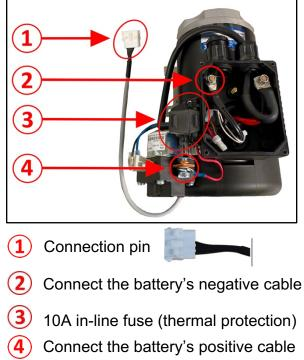
(do not forget to install the fuse holder)
