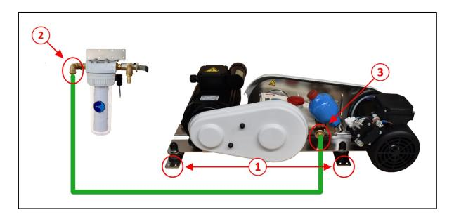
1: Stainless steel legs for fixing the motor/pump block
